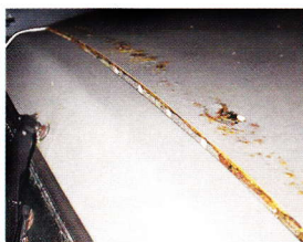
Estate CXs can rust along roof above hatch
