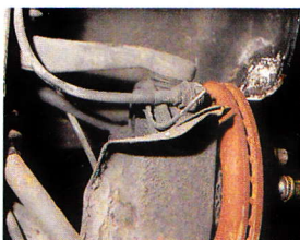
Upper ball-joint needs special extractor
