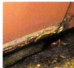
Crusty door bottoms typical of old CX
