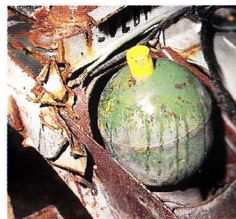
Gas-filled spheres need charging
