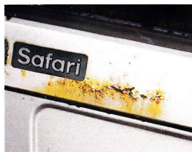
Watch for rust bubbling on the rear hatch
