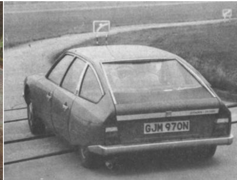
Above: Rear view emphasizes shrouded rear wheels and concave, sloping window. Boot opening extends down to bumper level
