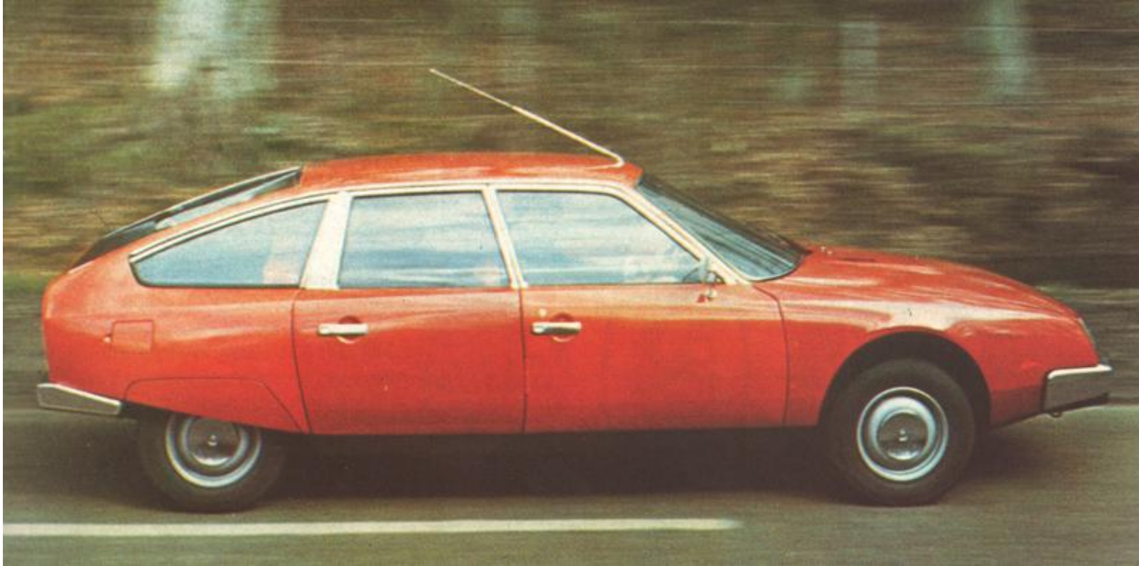
Above: Side view best shows true aerodynamic shape of Citroën CX
