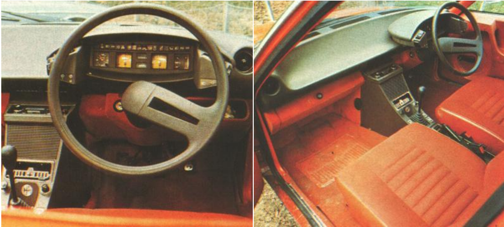
Above: Interior design includes futuristic "flying saucer" instrument and minor control binnacle. Single-spoke wheel is in true Citroën tradition
